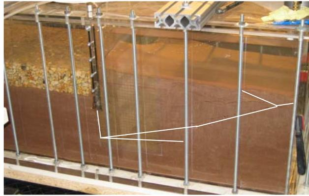
Figure 8. Result after failure (white line = slip plane)
